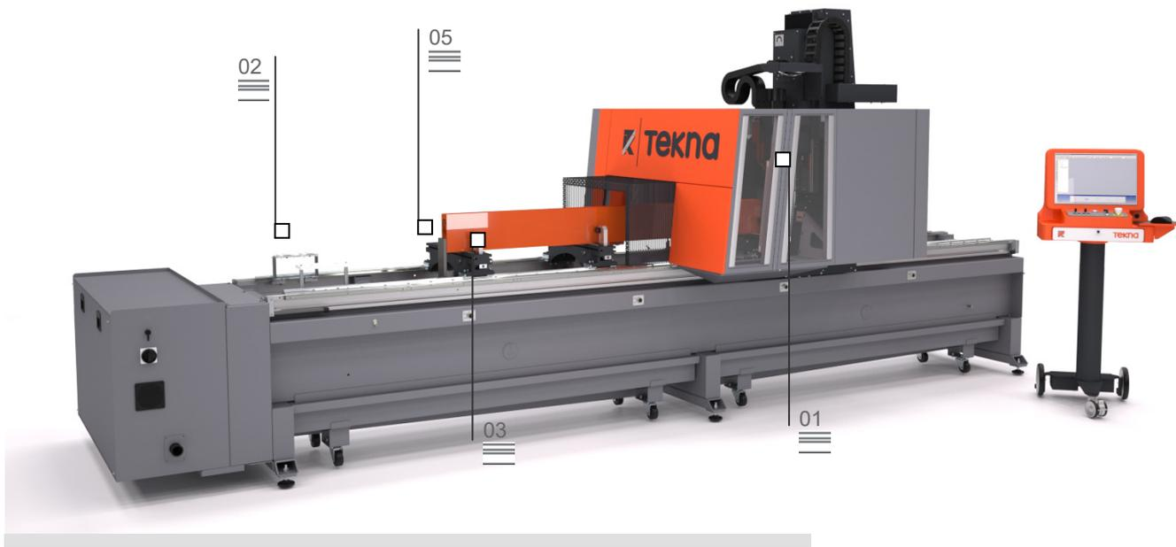
Mobile gantry CNC 4-axis machining centre, designed for drilling, milling and threading at any angle from  $-90^{\circ}$  to  $+90^{\circ}$  on bars or pieces in aluminium, PVC, light alloys in general and steel. The mobile part of the machine mainly consists of a gantry equipped with precision motorisation rack. The 8.5 kW electrospindle with ISO 30 tool connection is able to perform even heavy-duty machining with excellent, rapid and accurate results.
